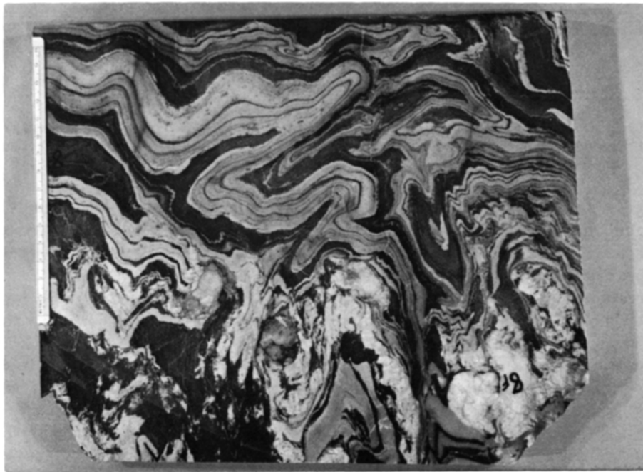
Fig. 1. Photograph of one level of the analyzed sample, measuring approximately 20 \times 30 cm. Notice the refold patterns in the upper portion of the sample and the complexities associated with the quartz-feldspar boudins in the lower portion.
